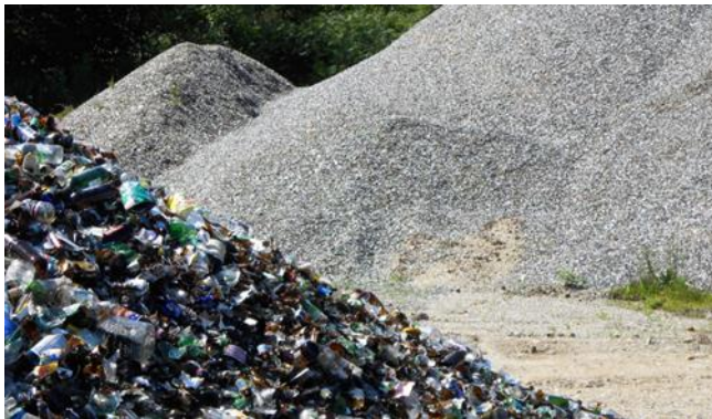
Glass before and after crushing into PGA
